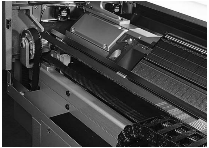
Large Knitting Machine (SUPER TORQUE Timing Belt)
